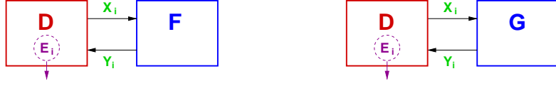
Fig. 5. Distinguishing two (\mathcal{X}, \mathcal{Y}) -random systems \mathbf{F} and \mathbf{G} by means of a distinguisher \mathbf{D} . The figure shows the two random experiments under consideration.
