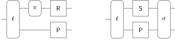
Figure 4.3: The real (left) and the ideal (right) setting considered in the context-restricted construction notion for a specific context (\mathbf{f}, \mathbf{P}) consisting of the filter \mathbf{f} and the auxiliary parallel resource \mathbf{P} .
